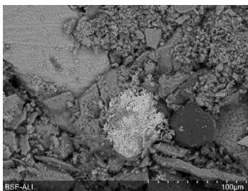
Figure 2. SEM of hydrochar formed from automotive fluff in the NRC-hydrothermal continuous system.
