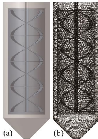
Fig.1 Diagram of (a) digester; (b) meshing of the physical model
