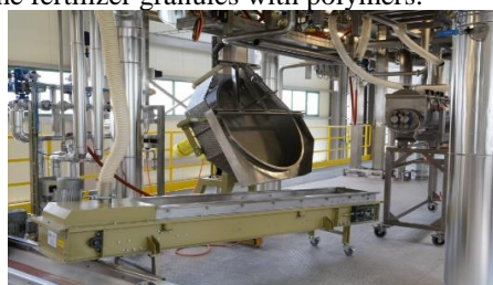
Fig. 2. Granulation unit of semi-pilot plant at Research Centre at Ł-INS
