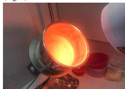
Fig. 4. Laboratory unit for coating granulated fertilizers with a Teflon covered drum and an infrared radiator (150W)
