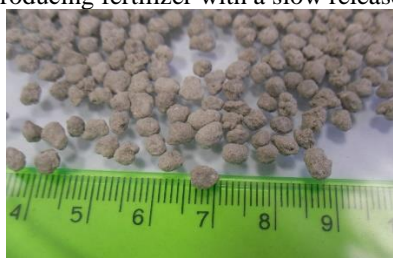
Fig. 1. Photograph of the adduct obtained in the semi technical plant test in 2011
