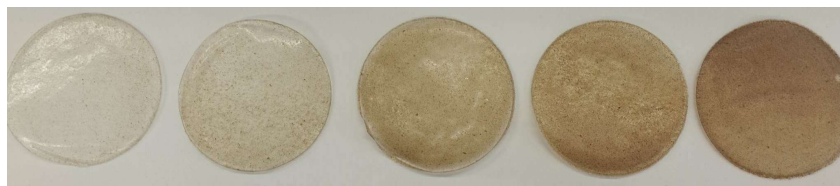
Figure 1. PLA based composite films with 2.5, 5, 10, 15 and 20 wt% of silverskin.
