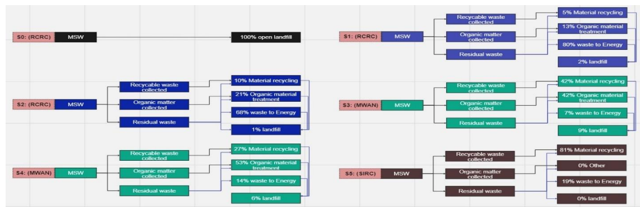
Figure 1. Municipal solid waste (MSW) management systems based on the proposed scenarios under study in Riyadh. (a) Scenario 0 (S0), (b) scenario 1 (S1), (c) scenario 2 (S2), scenario 3 (S3), scenario 4 (S4), and scenario 5 (S5).
