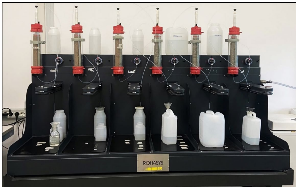
Figure 1 Picture of the experimental set-up employed to carry out the percolation leaching tests.
