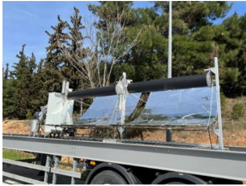
c) HTL reactor and in-house solar simulator setup; b) Solar simulator integrated HTL reactor during operation; c), d) Pilot-scale mobile HTL reactor with parabolic troughs
