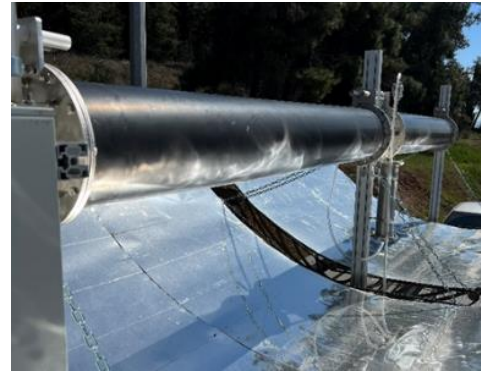
c) HTL reactor and in-house solar simulator setup; b) Solar simulator integrated HTL reactor during operation; c), d) Pilot-scale mobile HTL reactor with parabolic troughs
